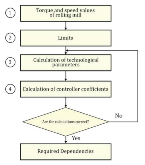
Generalized algorithm (control system module of an electric drive)
