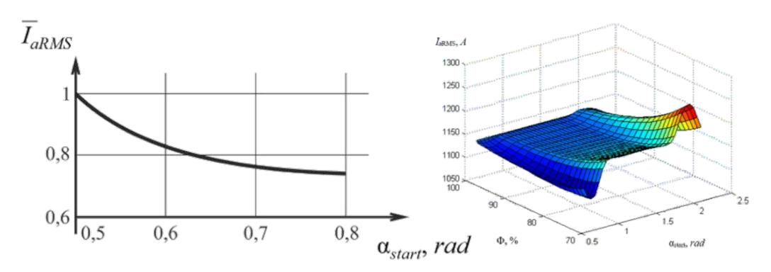
Calculation of the armature current rms value of a DC motor for a duty cycle.
