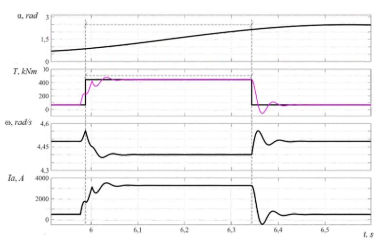
Electric drive dynamics (rolling mill electric drive)
